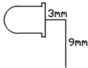
Position the front panel on to the case and drop it into place, making sure that the LED leads are inserted into their matching holes on the PCB. Once the panel is in place solder the LED leads **from the top of the PCB**.
